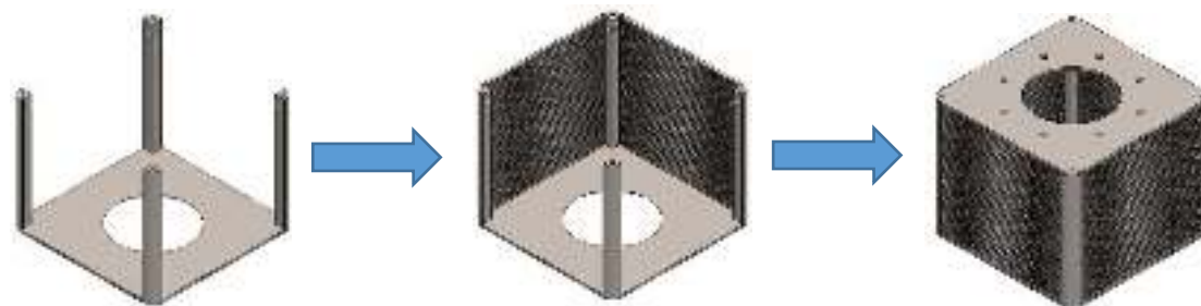
Figure 43 - The first iteration of the multi-component Faraday Cage design concept.
