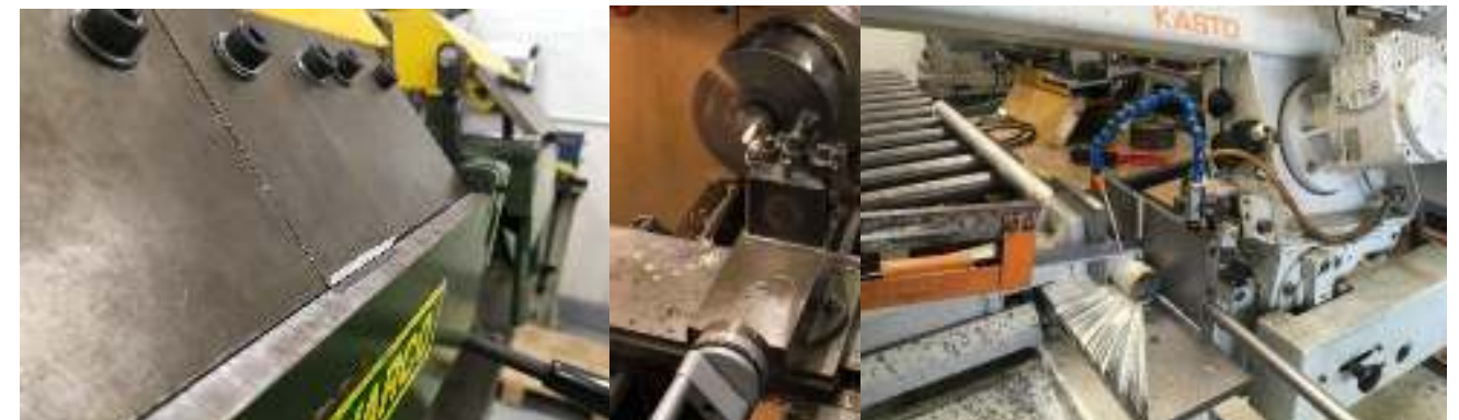
Figure 53 - Left to right: Folding the PTFE sleeves, lathing the PTFE rods, manufacturing an alternative testing anode.
