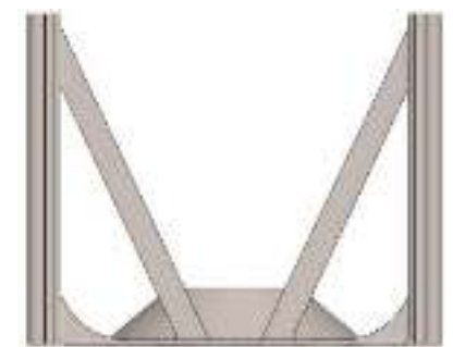
Figure 45 - Side profile of Faraday Cage base, showing the struts and 'nozzle.'
