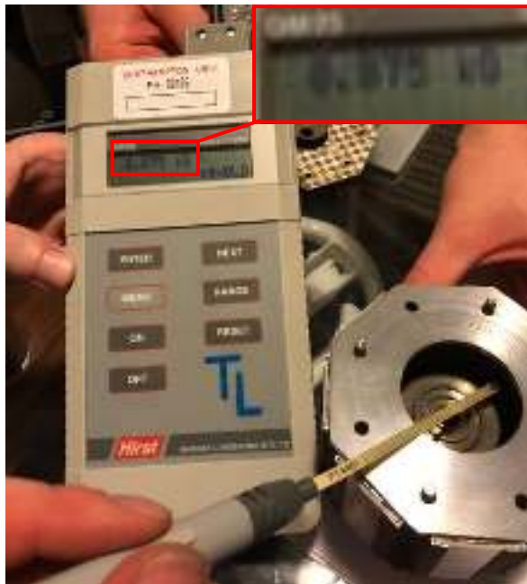
Figure 58 - Verification of the Magnetic Field Topology
