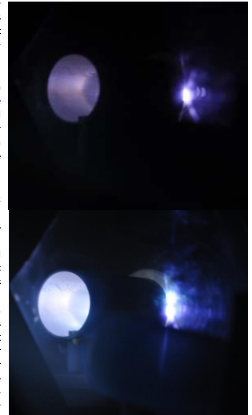
Figure 66 - A change in colour observed during testing with the cylindrical anode
