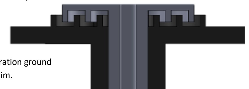
Figure 42 - SolidWorks cutaway of the Antenna Shield
