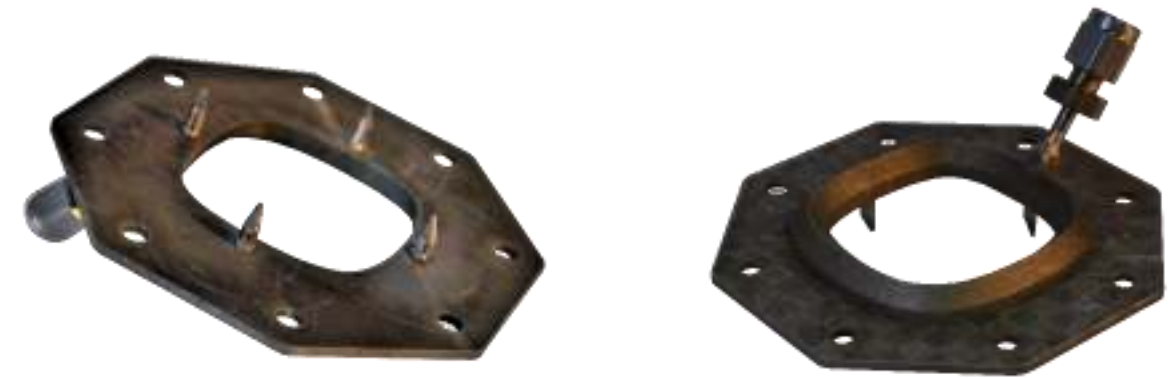
Figure 22 - The 4 propellant nozzles fixed to the reservoir plate.
