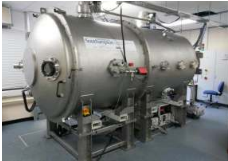
Figure 54- Large Vacuum Chamber in the David Fearn Electric Propulsion Laboratory
